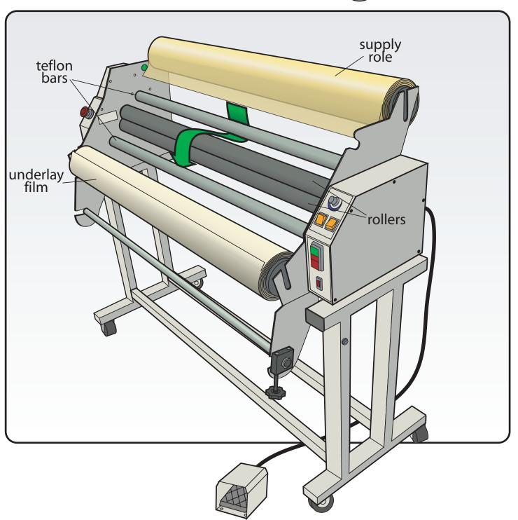
Take the ends of the bottom roll weave it under the Teflon bar pull the sheet toward you, grabbing all the way on each end. This time, pull out enough to stick firmly to the material from the top bar
