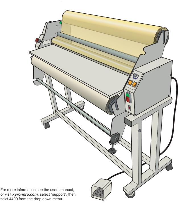
Remove media supporter before loading laminate rolls.
