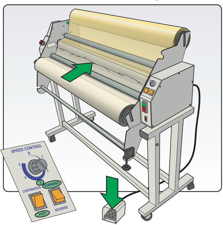
To remove the wrinkles from the material, press the foot pedal and use the load plate, or a scrap piece of cardboard and feed it through the machine until the wrinkles disappear.
