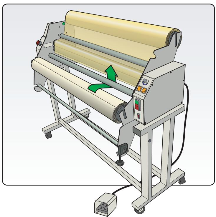
Using the foot pedal (direction, FORWARD; feed' FOOT; speed control, 3) start feeding it through so you can see about 3" coming out between rubber rollers in the back.
