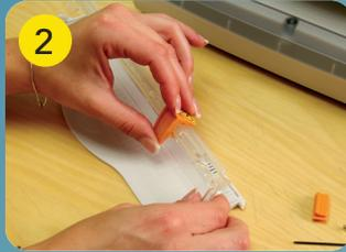
Carefully slide new blade onto cut bar. Note: Sharp edge of blade should be facing the machine. Replace the colored plastic insert and secure with wrench.
