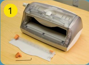
Loosen and remove the screw in the cut bar with wrench. Remove colored plastic insert and slide the old blade off cut bar (safely discard old blade).
