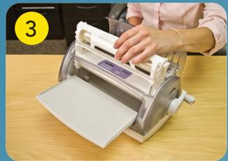
Open lid. Slide cartridge down into tracks on machine sides with exposed roll of material facing open lid cover. Close lid securely. Advance laminate and trim.
