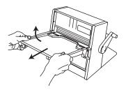
Remove used supply cartridge by pulling outward. If there is film between the rollers, turn handle counter-clockwise.
