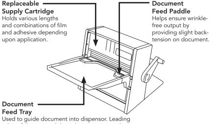
Used to guide document into dispensor. Leading edge of document slides in between tray and paddle during insertion. Align to right for A3/A4 documents, to the left for letter documents.
